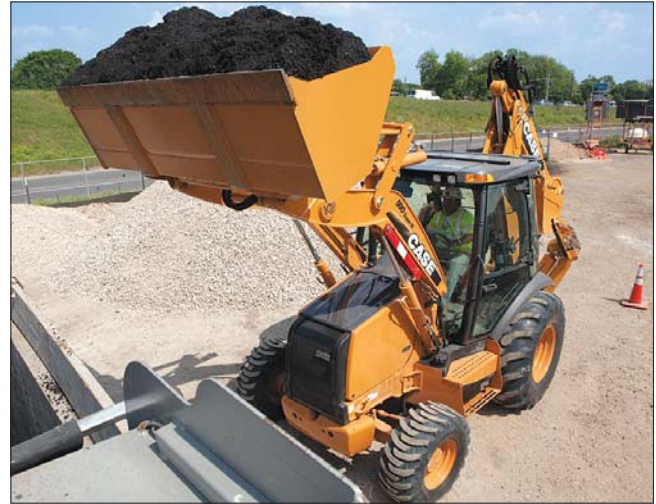
The Case N Series machines feature increased loader breakout and lift. The redesigned loader arms are stronger and longer, enabling the bucket to dump into the center of a truck for more efficient loading.
