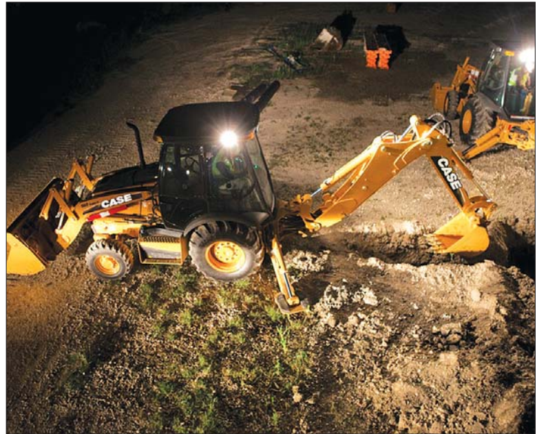
Side lighting on the new N Series loader/backhoes boosts safety and productivity in low-light conditions. Exterior lighting on the N Series machines includes two 55W halogen front driving lights, along with three sets of two adjustable 55W halogen work lights on the left side, right side and backhoe side of the cab canopy.
