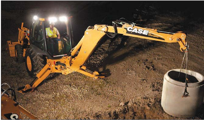
Power Lift delivers backhoe lift capabilities equivalent to a 5.5 ton (5 t) excavator and the dig depth of an 8.2 ton (7.5 t) excavator.
